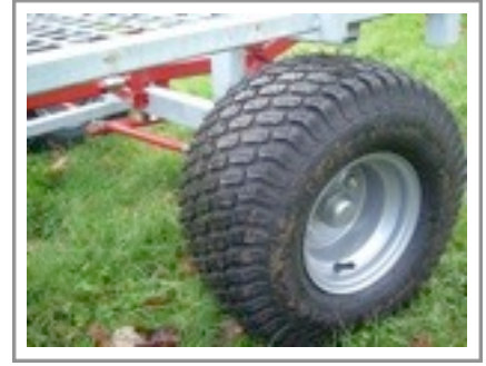
Wheels: 6-ply tyre's, 800 x 5 highway tread with taper roller bearing hub. 18"
