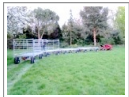
Wheels: 6-ply tyre's, 800 x 5 highway tread with taper roller bearing hub. 18"
