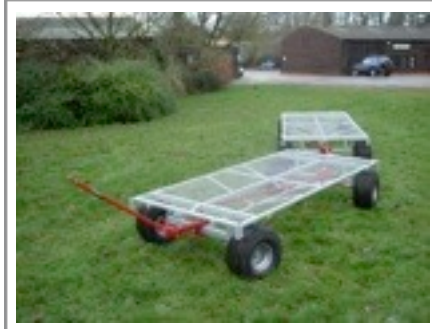
Pulls from either end by changing towing handle to opposite end of trolley.
