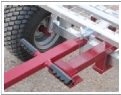
Double Ackerman steering (for greater stability with the 8' x 4') ensures good following for multiple towing.
