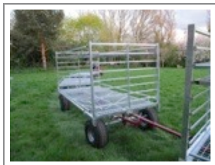
Double Ackerman steering (for greater stability with the 8' x 4') ensures good following for multiple towing.
